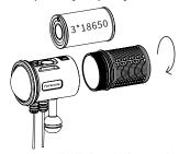
Step 3: Power on - Press and hold both switches for 3 seconds to turn it on The default maximum nower (9th mode) is 8000 lumens. Step 4: Dimming - The left button is for downshifting and the right button
